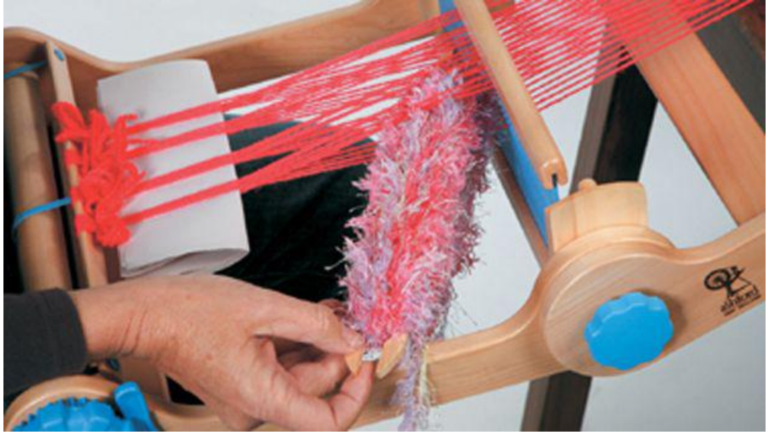
The shuttle is passed through the open space between warp yarns to create fabric.
